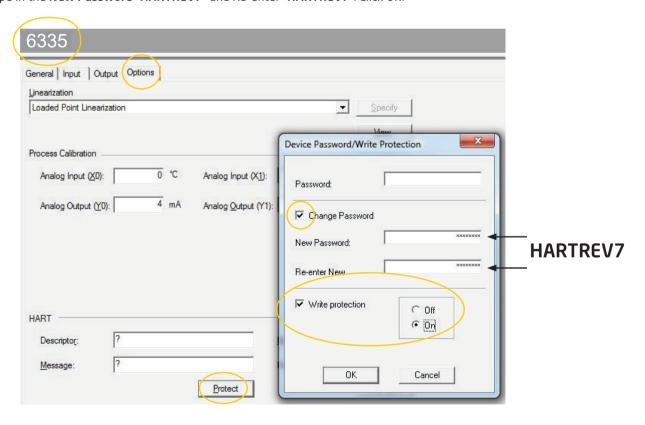
Switch **Write protection OFF** and write-enable the device by typing in the **Password** "-**CHANGE-**" in the top menuacknowledge by pressing OK.
